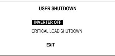
The Operator can invoke two types of shutdowns from this interface screen:
